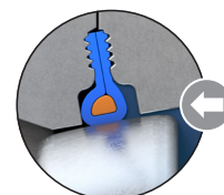
Disc in Closed Position. Line pressure applied from the non-preferred flow direction.
